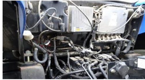
Nav controller mounted outside cab
